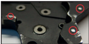
14. Grind pins in red circles to fit wires into the gearbox.
