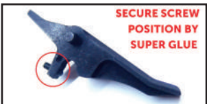
19. If you want shorter trigger path, insert screw into the trigger. After testing secure its position by super glue.
