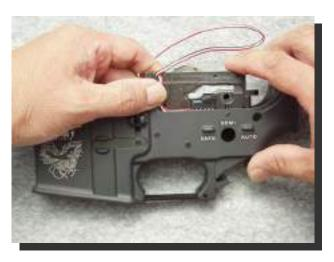
Once the gearbox is fully seated into the lower receiver, secure the gearbox by fastening two Set Screws for Gear Box (GB-025) through the mounting holes of the gearbox, onto the lower receiver.
