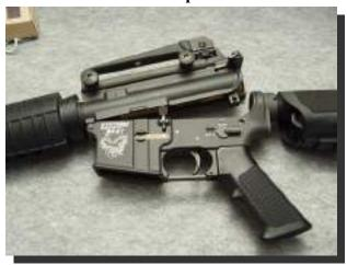
During installation, if you have to hammer the pin in place, make sure the holes in the upper/lower receivers are perfectly lined up first to avoid damage to the receiver.
