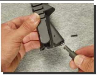
Once the groove is aligned inside the receiver, insert set pin from below the receiver. The pin is easier to install from below with the receiver upside-down because the receiver sits more securely this way.
