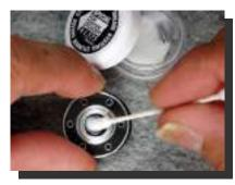
Place Piston Head Guide Spring (CU-013) over Piston Head Guide (CU-014), and insert the piston head guide through the opening in the piston as shown. While pressing the piston head guide through the opening (the spring should not protrude), apply glue to the thread and tighten piston head onto the piston head guide.
