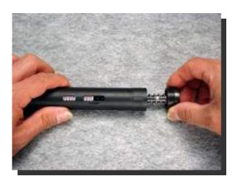
4. Install Inner-Barrel Assembly Insert Inner-Barrel Assembly (ASS-BR-04/05) to upper receiver, noting the orientation of the BB feeding opening, as shown.
