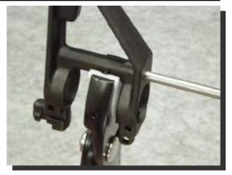
Insert front sight post over barrel. The gas pipe should pass through the corresponding hole in the hand guard cap, barrel nut assembly (hole prepared in last step), and finally into the upper receiver.
