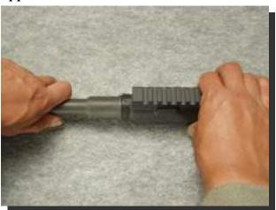
From the front of the outer barrel, screw in Barrel Nut Assembly (ASS-BR-03). The barrel nut assembly consists of 4 parts (barrel nut, slip ring, weld spring, and ering). To properly install the gas pipe later, the notch / holes on these 4 parts and the hole in the upper receiver must align properly. Use a tool such as small screw driver to ensure proper alignment.
