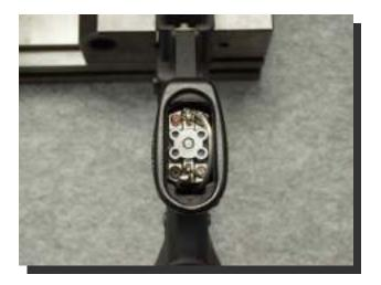
Once the grip is fully inserted, through the opening at the bottom make sure the positive motor wire is routed towards the side of the motor's bottom mount point. There is a small notch on either side of the grip end for the wire to rest. If the wire do not rest in said groove, it will be damaged.
